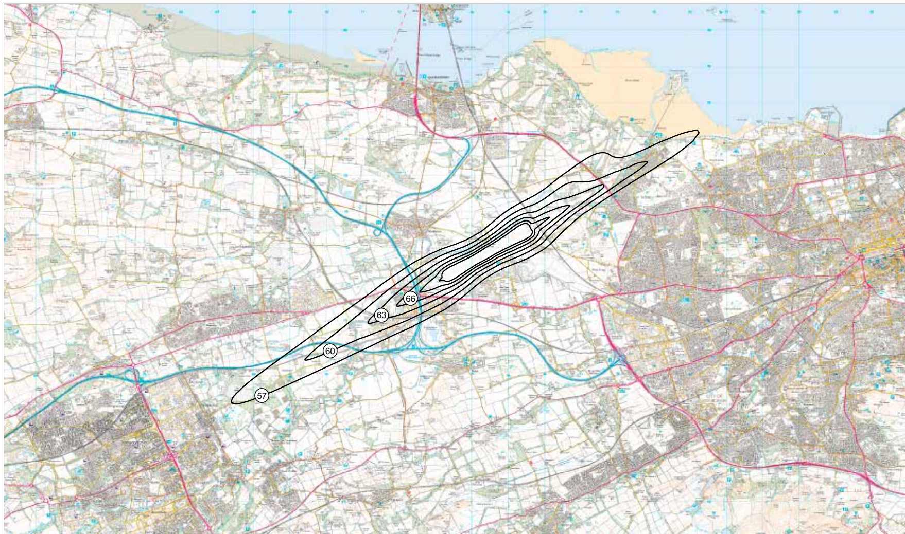
EDINBURGH AIRPORT 2016 Annual Day L_{Aeq,16hr} 57-72 dB(A) Contours Actual Modal Split 68% W / 32% E
